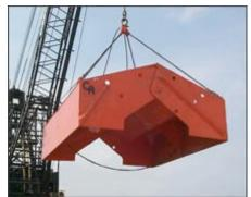
As required by the project specifications, dredging will be conducted using an eight (8) cubic yard environmental clamshell bucket manufactured by Cable Arm. The Cable Arm clamshell bucket's lightweight design enables only soft sediment to be removed.
